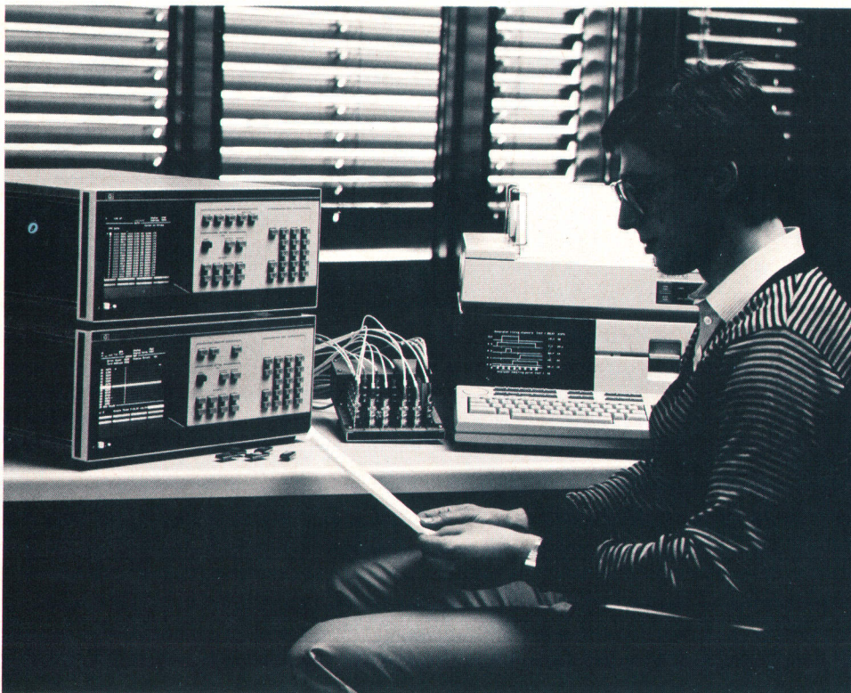
Fig. 1. The 8180A Data Generator (top left), the 8181A Extender (not shown), and the 8182A Data Analyzer (bottom left) provide high-performance, easy-to-use, economical at-speed testing for digital integrated circuits, boards, and modules. The system can be controlled by a desktop computer (right) via the HP-IB (IEEE 488).
