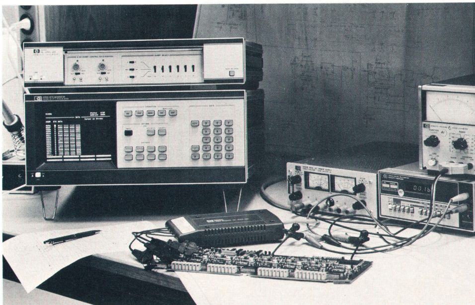
Fig. 9. The tri-state pod makes the data generator outputs compatible with bidirectional bus and I/O pin configurations. The control and power unit on top of the 8180A Data Generator is part of the pod system.
